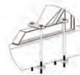
Position mounting bracket over gusset
